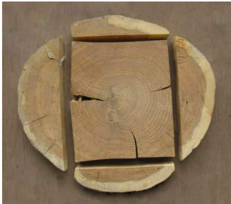
Figure 24: Cross section of a boxed heart timber. (Photograph courtesy of Joe Thompson.)
