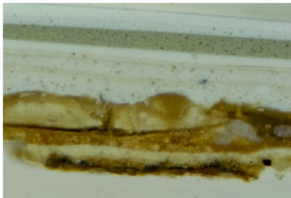
066 East wall cornice, flaking paint vis. 125X
