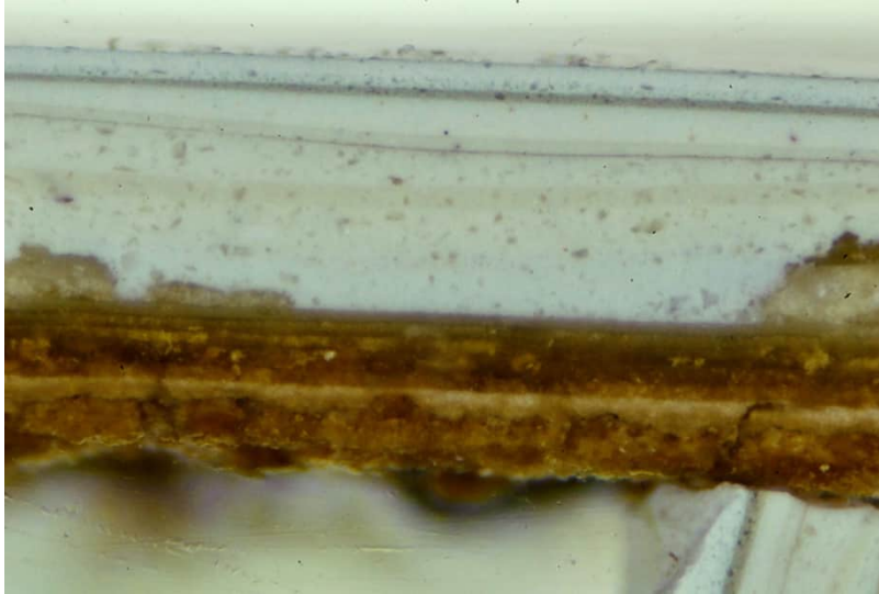
071 East wall cornice behind removed cupboard, NE corner vis 50 X
