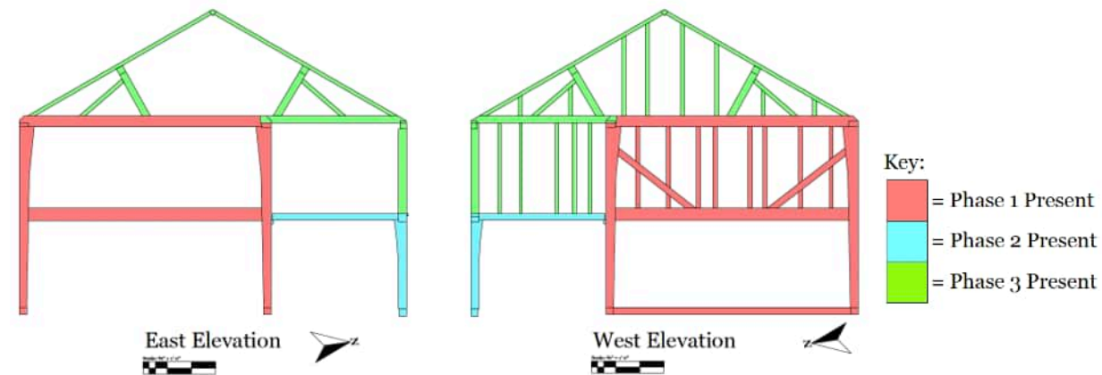
Figure 58. Phase 3, east and west elevations showing the principal framing elements by phase which exist in 2026. Where studs are not drawn indicates that the framing was not accessible in those areas. Where sills are not drawn indicates that they have been replaced since the Phase 3 construction. (Drawing by Nevan Carling.)
