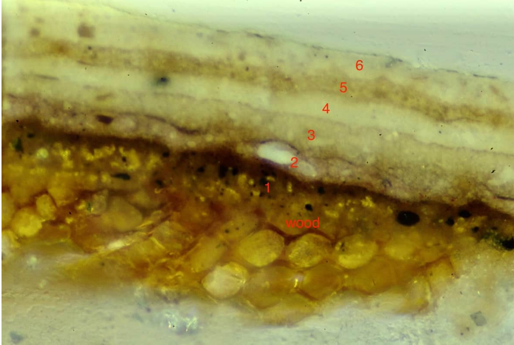
Figure 44. Photomicrograph of paint sample NPH 006 taken from the wainscot on the north wall which was not covered by the door architrave during Phase 3 or early Phase 4. This sample shows 4 layers of the tan yellow, but without any significant dirt line between layers, suggesting that the interval of time between applications was not particularly long. Numerous paint layers were applied after layer 6, but these were stripped in the 3 rd quarter of the 20 th century. (Photograph by Christine Thomson.)
